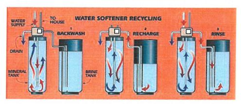
The back wash phase removes hard water deposits from the mineral tank.
